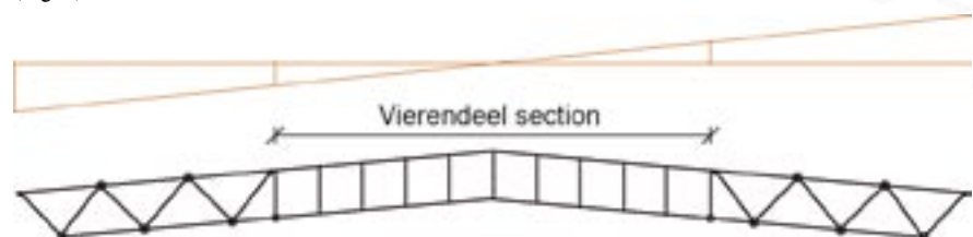
Fig. 1: Transverse force distribution across a single-span girder
